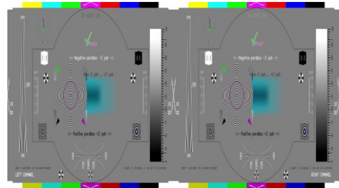
VQ MPC-AVS: Multi-Purpose Dynamic Chart with AV Sync component, versions up to UHD, 16 bit per component
